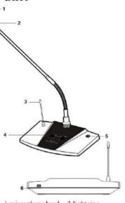
1,microphone head 2.light ring 3.transmit antenna 4.LCD screen 5.power switch 6.USB charge interface
